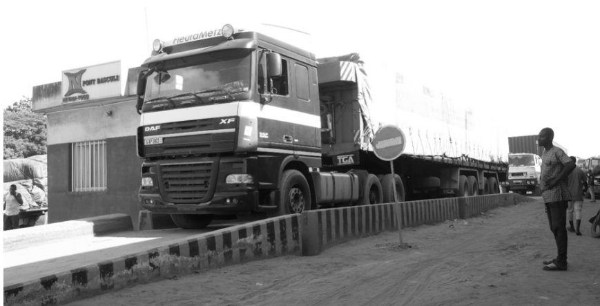
Figure 8. A trailer truck mounted on a weighbridge weighing ferrous scrap
